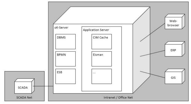
• Standard Customer Environment - there is not standardized way, how DSO are splitting up resources on multiple hardware components (see following image for a possible scenario)
