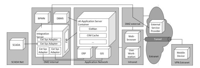
It is possible, that the SCADA System has access to the integration server, but not the other way around.
