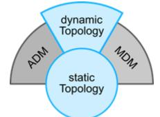
The figure above shows the dependencies between the described Domain Modules ADM, MDM and TDM. The TDM (blue) consists of two services. The core-service provides static topological-information about the installed conducting equipment. This information can be used by the second TDM-service (dynamic Topology), that uses the current switch- and tap-changer-states, to enable the view on the current electrically connected power grid. The
