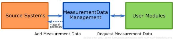
The MeasurementDataManagement might use Core Modules in the future for tasks such as authentication/authorization, logging, and technical monitoring.
