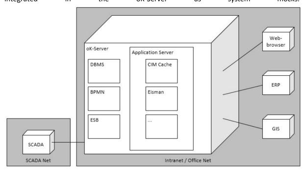
Standard Customer Environment - there is not standardized way, how DSO are splitting up resources on multiple hardware components (see following image for a possible scenario (DEPRECATED as going for microservices))
