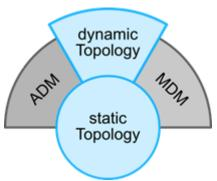
The figure above shows the dependencies between the described Domain Modules ADM, MDM and TDM. The TDM (blue) consists of two services. The core-service provides static topological-information about the installed conducting equipment. This information can be used by the second TDM-service (dynamic Topology), that uses the current switch- and tap-changer-states, to enable the view on the current electrically connected power grid. The
