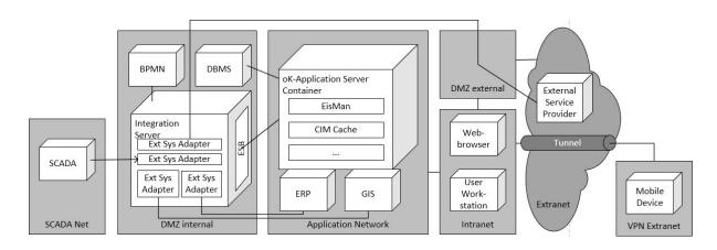
It is possible, that the SCADA System has access to the integration server, but not the other way around.
